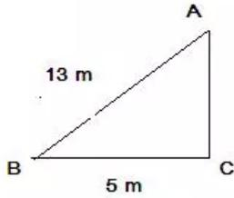
Pythagoras theorem states that in a right angled triangle, the square on the hypotenuse is equal to the sum of the squares on the remaining two sides.
