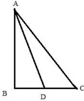
Pythagoras theorem states that in a right angled triangle, the square on the hypotenuse is equal to the sum of the squares on the remaining two sides.
