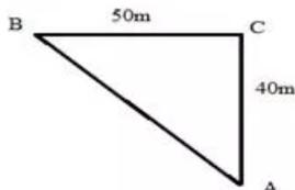
Pythagoras theorem states that in a right angled triangle, the square on the hypotenuse is equal to the sum of the squares on the remaining two sides.
